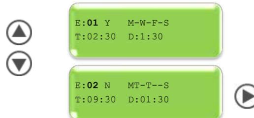
**Priming the pumps:** Hold down the up ^ arrow until the chemical reaches the injection point.
