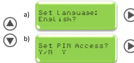
**Step 2:** If you selected 'Y=Yes' set a unique 4 digit PIN to enable unwanted access (a). Now confirm the pin entered with Y/N? (If 'N=No' is selected you will need to repeat steps 1&2).
