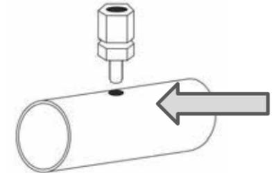
**Step 2:** For added security it is recommended to use Silicone Sealant (not-supplied) in-between the Pipe Injector and the drilled hole (as shown above). Slowly wind in the Pipe Injector until tight, it is not necessary to over tighten with tools as this may damage the threading on the injector.
